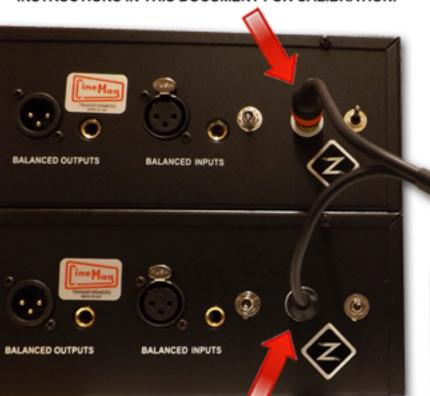
PLUG THE RCA CABLES INTO THE REAR OF EACH UNIT AND INTO THE STEREO LINK BOX.
