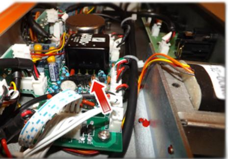
PLACE NEW JOHN HARDY OP-AMP IN THE EMPTY SLOT AND MAKE SURE PINS ARE LINED UP CORRECTLY
