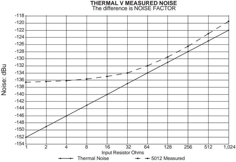
A graph can be drawn showing Noise against Resistance. Thermal, or pure Resistor noise is a straight line whilst Amplifier noise is a curve that depends upon the optimum source resistance for that particular amplifier. The difference between the two noise measurements in dB is the “Noise Factor”. (“N.F.” Familiar to R.F. and communications designers.)
